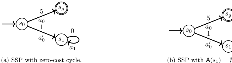
Figure 2: SSPs that violate assumption 2, and consequently have optimal value functions that induce suboptimal policies. One SSP violates it with a zero-cost cycle, and the other SSP violates it by having a state with no applicable actions.
